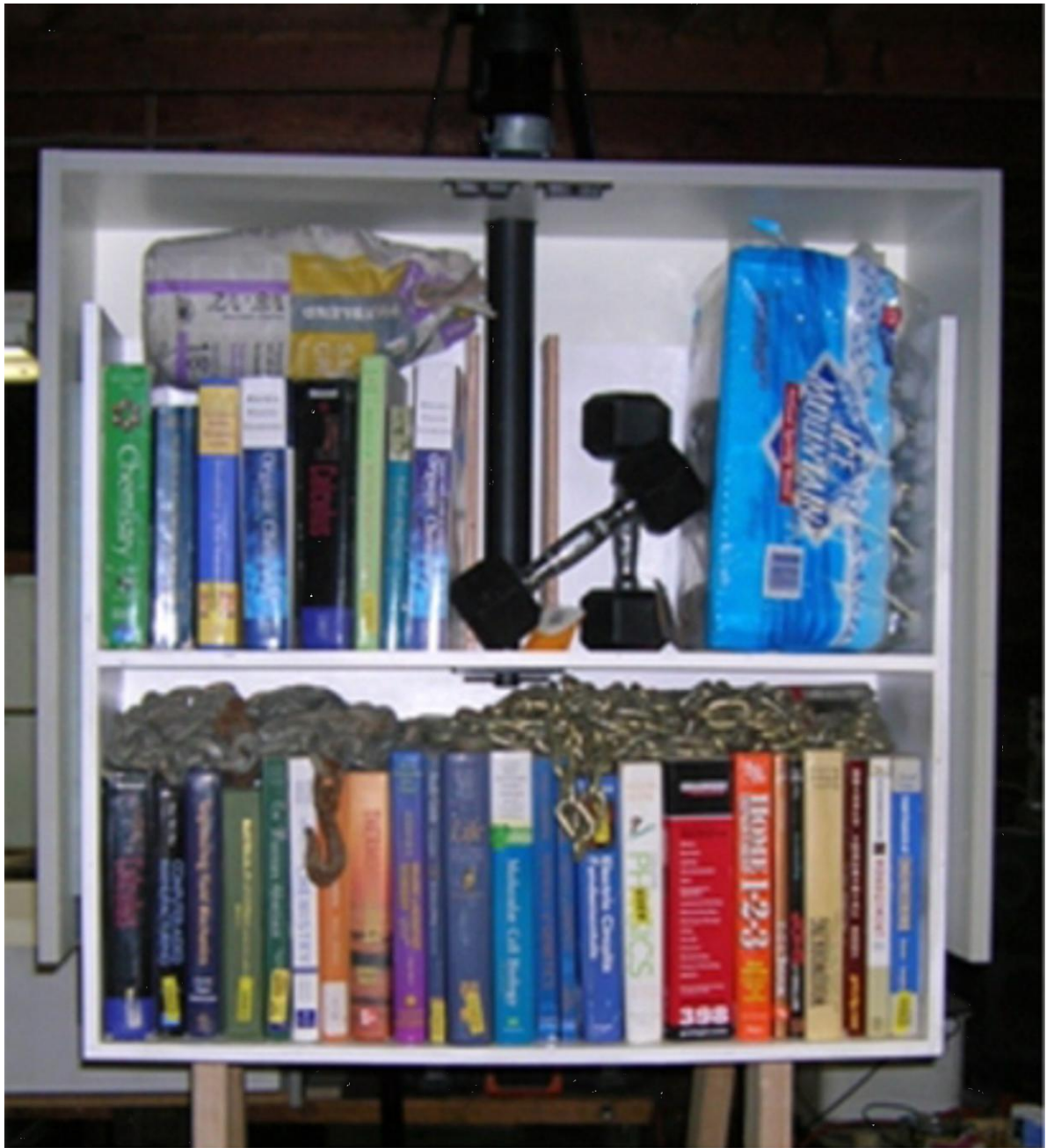
Fig. 18.21. Modified Cabinet During Testing.
